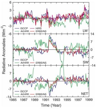
FIG. 6. Time series of deseasonalized tropical mean (20°N to 20°S) broadband radiation budget anomalies (LW, SW, and net) from 1985 to 1999 from the ERBS Nonscanner WFOV Edition3\_Rev1 (red), ISCCP FD (blue), HIRS Pathfinder OLR (pink), and AVHRR Pathfinder ERB (green) data records. Anomalies are defined with respect to the 1985 to 1989 period.
