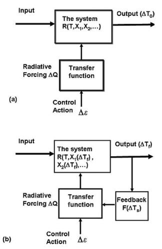
FIG. 10. (a) The main elements of an open (energy balance) climate system, where X is independent of output  $\Delta T_o$ . The climate forcing involves the transfer function mapping from the control action to a change in radiative budget. (b) The control action modulates the output  $\Delta T_f$  and feedback is established by a loop connecting the output to input.
