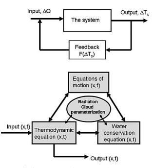
FIG. 2. (top) The common, simple system view of the globalmean climate system with feedbacks. (bottom) A view of one component of the climate system expanded for detail indicating the set of connecting subcomponents, each composed of processes that couple to other processes in space (x) and time (t).
