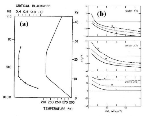
FIG. 9. (a) The critical-blackness cloud experiment of Manabe and Strickler (1964). The profile to the left is the profile of emissivity above which clouds warm the surface relative to the given clear-sky temperature profile (right). (b) The change in equilibrium surface temperature as a function of cloud LWP and IWP for low (L), middle (M) and high (H) clouds (Stephens and Webster 1981).
