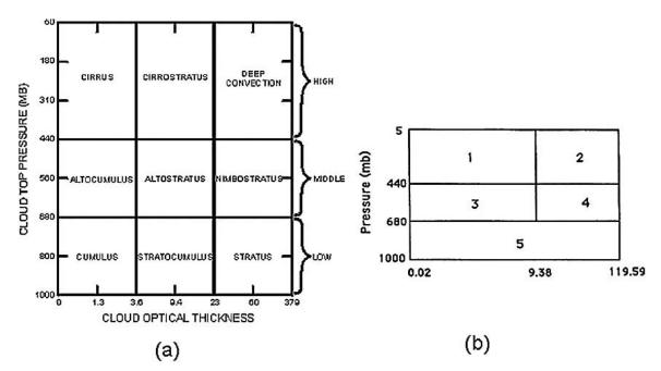
FIG. 8. (a) The radiometric classification of cloudy pixels in terms of optical depth and cloud-top pressure according to ISCCP. (b) The reduced set of five cloud types of OBH.
