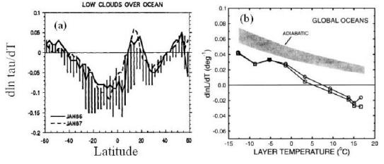
FIG. 11. (a) The local sensitivity of cloud optical depth derived from ISCCP with cloud temperature (Tselioudis and Rossow 1994). (b) The local sensitivity of cloud liquid water path derived from SSM/I microwave radiance data with cloud temperature (Greenwald et al. 1995).
