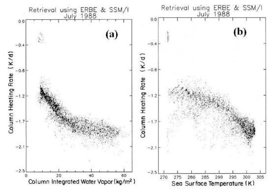
FIG. 12. (a) The relationship between longwave component of  $R_{\text{atm}}$  and column water vapor. (b) Same as in (a) but for SST (from Stephens et al. 1994).
