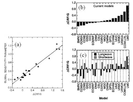
FIG. 14. (a) The global sensitivity parameter as defined by Cess for the  $\pm 2$  K SST perturbation experiments plotted as a function of the ratio of the change in  $C_{\text{net}}$  to change in net radiation budget for 19 GCMs. (b) This ratio derived from updated group of models in the Cess et al. (1996) update. (c) The breakdown of long- and shortwave components of the ratio.
